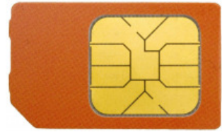
Fig. 12.21 GSM SIM card
