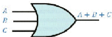
Fig 2.7 : OR gate with three inputs
