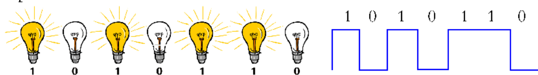
Fig. 2.2 : Digital representation of ON and OFF
