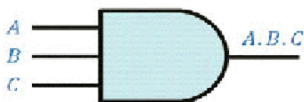
Fig. 2.10 : AND gate with three inputs
