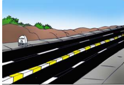
Median divides a road into two equal parts
