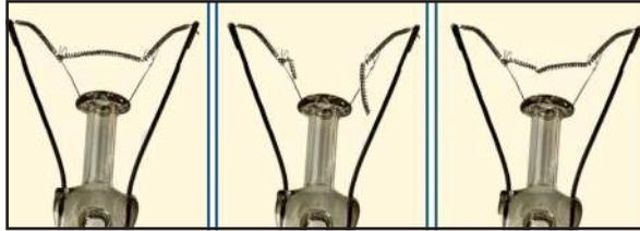
If a bulb is lit after rejoining the parts of a broken filament, what change will occur in the intensity of the light from the lamp? What will be the change in the power of the bulb?
