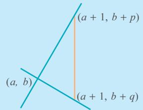
Since the lines are perpendicular, the points  $(a, b)$ ,  $(a + 1, b + p)$ ,  $(a + 1, b + q)$  are the vertices of a right angled triangle. The hypotenuse is the line joining the second and third points. So, the squares of the lengths of the perpendicular sides of this triangle are  $p^2 + 1$  and  $q^2 + 1$  and the length of the hypotenuse is  $|p - q|$ . This gives
