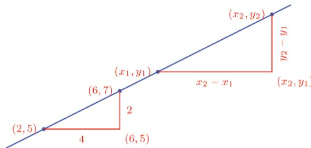
The perpendicular sides of the lower triangle are 4 and 2. That is, the vertical side is half the horizontal side. It must be so for the upper triangle also (why?) Thus
