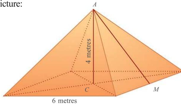
The slant height we need is  $AM$ . Joining  $CM$ , we get a right triangle with  $AM$  as hypotenuse. What is the length of  $CM$  in it?
