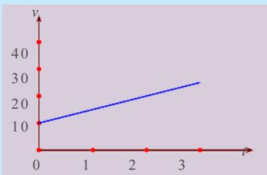
The slope of this line is 5. Here the slope is the rate at which  $v$  changes with respect to  $t$ ; that is, the acceleration.
