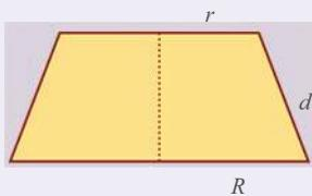
Taking the slant heights of the large and small cones as  $L$  and  $l$ , we get the  $d$  in the figure above as  $d = L - l$ . So the surface area of the frustum is,
