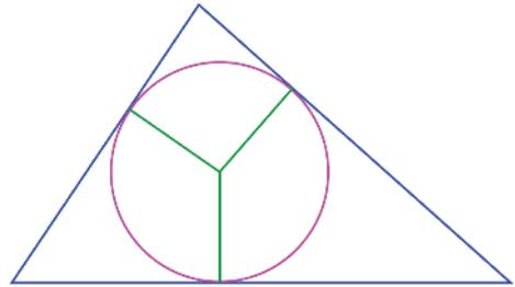
The sides of the triangle are formed by the tangents to the incircle from the vertices. And the lengths of the tangents from each corner are equal. So taking the lengths of the tangents as  $x, y, z$ , we can mark them as below:
