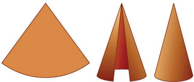
The radius of the sector becomes the slant height of the cone. The arc length of the sector becomes the circumference of the base of the cone.
