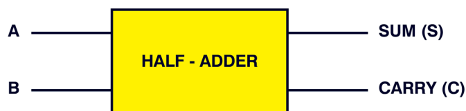
Fig. 10.29 Logic Symbol of Half-Adder
