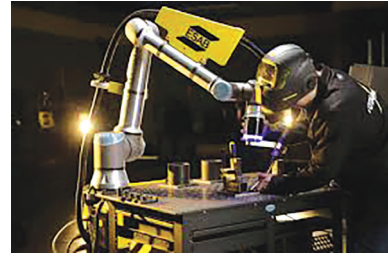
Fig. 11.10 : COBOT for welding
