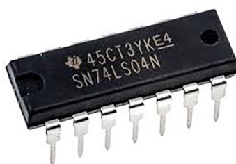
Fig. 6.31 IC- 74LS04 Pin diagram and package
