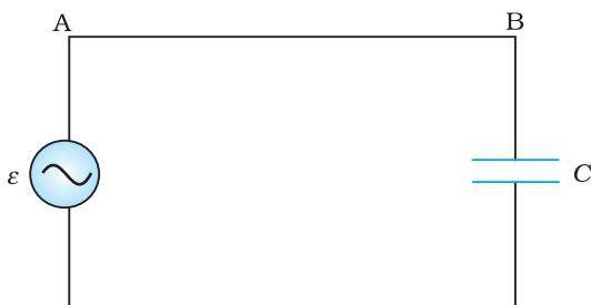
FIGURE 7.7 An ac source connected to a capacitor.
