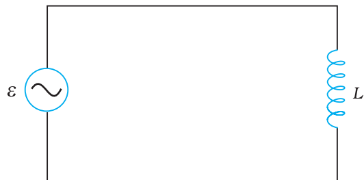
FIGURE 7.5 An ac source connected to an inductor.
